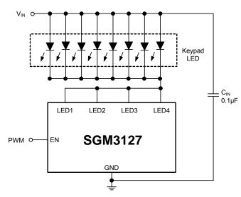
Figure 2. Application Circuit for Keypad
