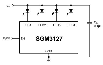
Figure 1. Application Circuit for Backlight
